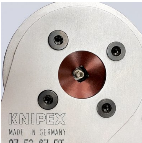
Synchronous feed of the four mandrels ensures optimum crimping result with 4/8 indent
