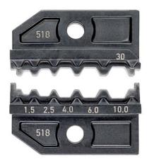
Application: non-insulated terminals in accordance with DIN 46235 and crimp connectors in accordance with DIN 46267 1.5 - 4.0 mm<sup>2</sup> and 6.0 + 10.0 mm<sup>2</sup>
