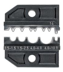
Application: for non-insulated crimp terminals, tube and compression cable lugs in accordance with DIN 46234 and DIN 46235 and noninsulated crimp, butt and press connectors in accordance with DIN 46341 and DIN 46267 0.5-10 mm²
