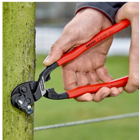
two-hand operation for maximum cutting force
