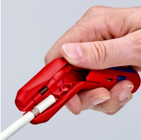
Stripping of a coax cable
