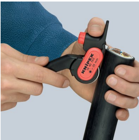
Setting the tool for longitudinal cut
