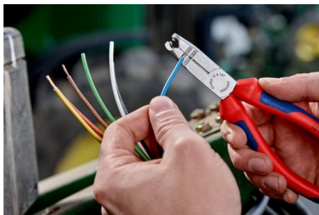
wire stripping holes for 1.5 and 2.5 mm 2 conductors
